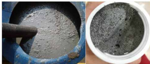
Figure 3—Significant amount of sand with proppants (2 barrels) was collected during desander flushing in August 2018.
