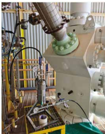
Figure 5—Online sand sampler (OSS) setup at wellhead area (upstream of the wellhead desander) to collect physical sand samples from the flowline by connecting to the sampling point.
