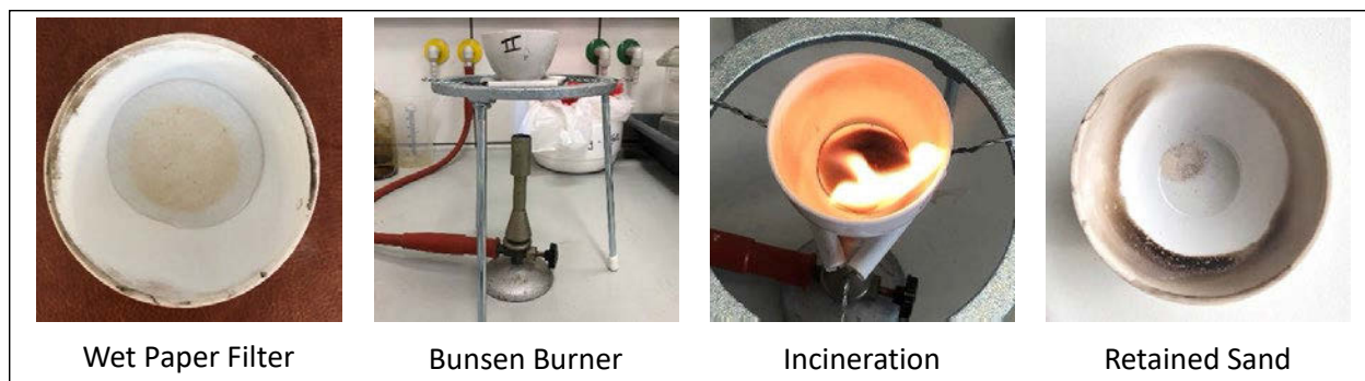
Fig. 6 Process steps of incineration
