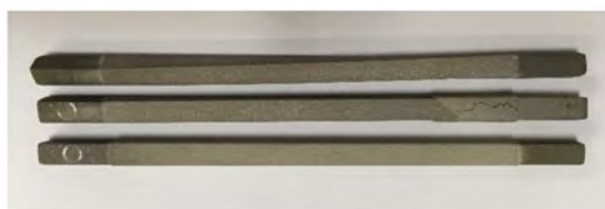
Figure 8—Coated steel rods after torsional experiments
