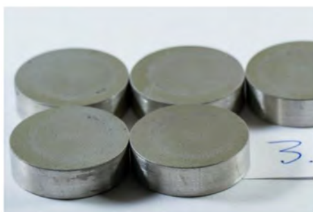
Figure 4—Coated Coupons before Corrosion
