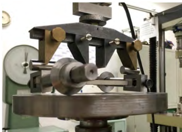
Figure 7—Apparatus for bending experiments
