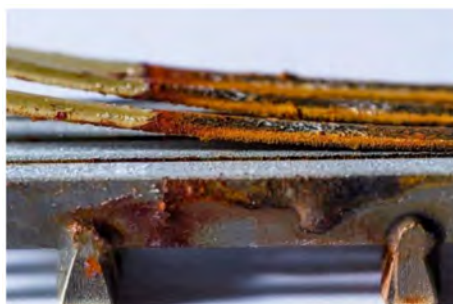
Figure 5—Example for a separation of screen and coating without the use of a bonding layer
